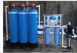
FRP RO Plant
