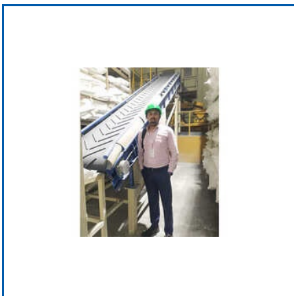
INCLINE BELT CONVEYOR
