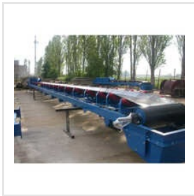
Rubber Belt Conveyor
