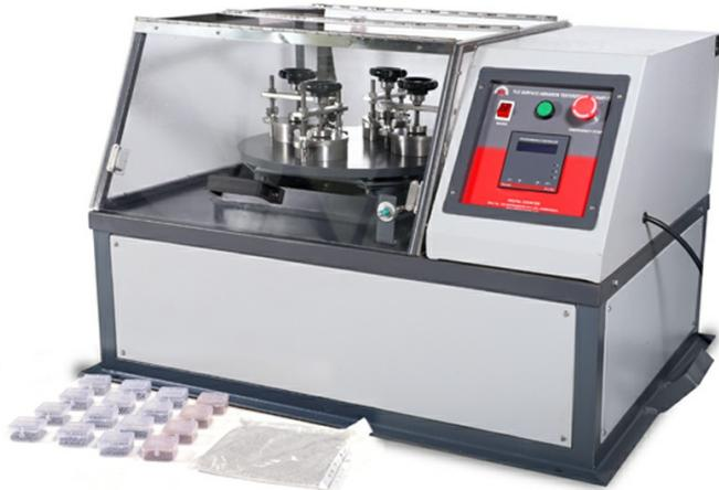
The test is conducted by holding a number of test specimens on a flat horizontal disc. The disc is rotated at a speed of 300 rpm with the axis of rotation 22.5 mm out. This causes the abrasive load placed above the test specimen to rub over the surface of test specimen in a circle of 45 cm diameter. The abrasive load is kept in place over the test surface inside a rubber lined cylindrical metallic ring. The ring also keeps the test specimen firmly pressed against the metallic disc.
