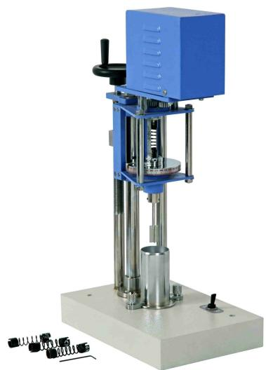
The Vane shaft is attached through the hollow upper shaft to re-settable pointer, which indicates the angle of torque on a dial graduated in degrees. The dial reading multiplied by spring factory gives the torque. A container for soil tube of 38mm I.D. & 150 mm long can also be used as container. Complete with set of springs, one each of approx 0.2 kg/cm, 4 kg/cm, 6 kg/cm, 8 kg/cm
