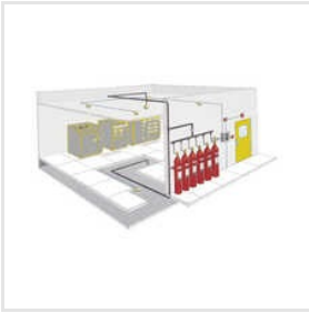
Fire Gas Flooding System
