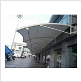
Outdoor Tensile Membrane Structure
