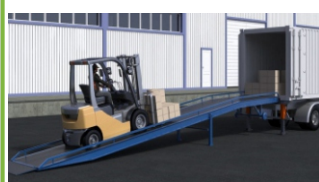
Mobile Loding Ramp
