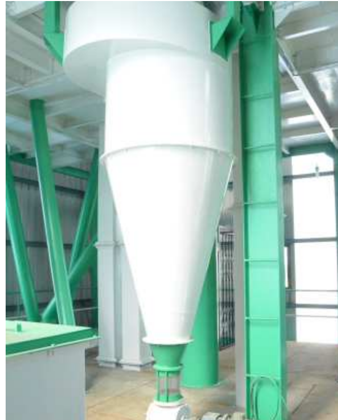
CYCLONE FOR SEPARATION OF FEED DUST AIR
