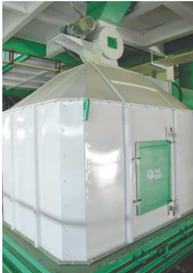
COUNTER FLOW PELLET COOLER MODELS AVAILABLE 1MT/HR. TO 30MT/HR.
