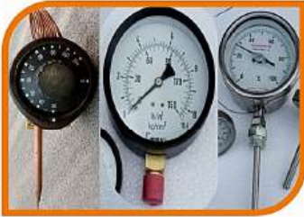
Pressure Switch, Pressure Gauge, Temperature Gauge
