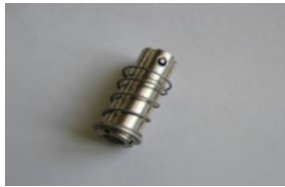
Plunger with fixed conical & cylindrical seal (Old Plunger) Photo – 4
