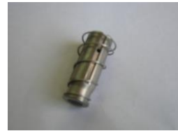
Plunger with moving seal (New Design Plunger) Photo – 5
