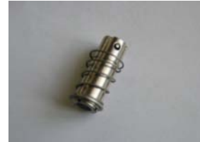
Plunger with fixed conical & cylindrical seal (Old Plunger) Photo – 3
