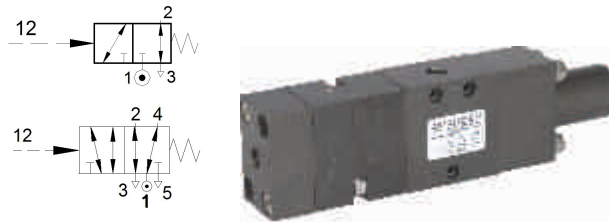
3/2, 5/2 Air Operated Spring Return Valve Low Pilot Pressure: 5 - 160 bar
