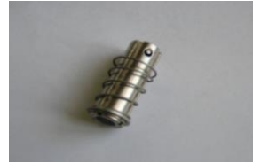
Plunger with fixed conical & cylindrical seal (Old Plunger) Photo – 3
