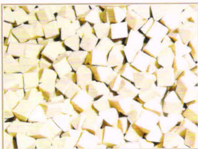
White Media: Use For Polishing 25% white alumina
