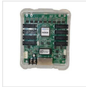
LED Controller Receiver Card Nova Star IND528
