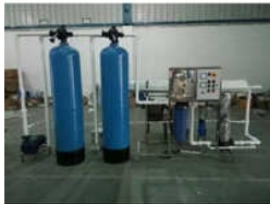
2000 LPH Industrial Reverse Osmosis Plant
