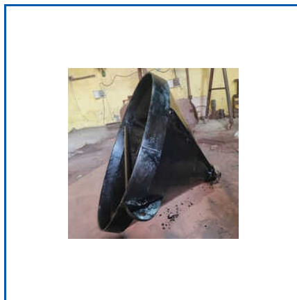
CONCRETE HOPPER (TREMIE PIPE)
