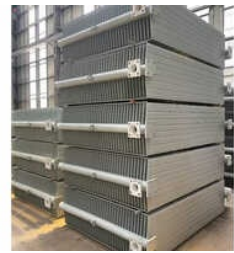
315 Kva 3 Phase Power Transformers Radiator
