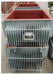
Distribution Transformer Radiator
