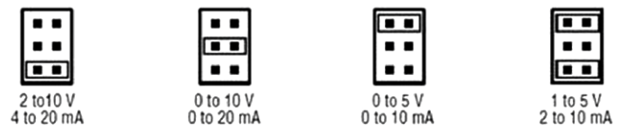
Figure 4: Output Range Selection Jumper (PJ5)
