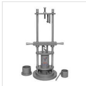
Aggregate Impact Testing Machine
