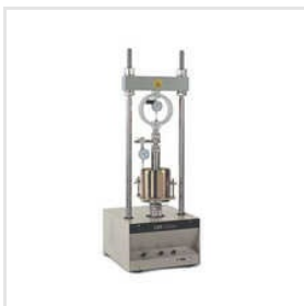
Laboratory CBR Apparatus
