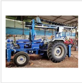
Tractor Fitted Piling Machine
