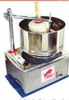
In this we can grind Vada, Batter, Masala, Chutney & Kurma and we can attach coconut scrapper for scrapping coconut Flakes/Flowers.
