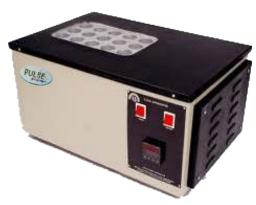
The PULSE DIGITAL COD DIGESTOR is suitable for COD method for monitoring waste water influent & effluent, industrial process water. Outer cabinet made of mild steel duly coated. Double wall construction with insulation for minimum heat losses increases the efficiency of the system. Aluminum Block with holes dimension is used to hold 15 nos. Selectable time up to 1230 min with alarm is provided to set the digestion period (Refluxing)
