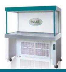
The PULSE Laminar Air Flow is designed to provide working space comprising as standard features HEPA filter having efficiency of 99.97% down to 0.3% microns, prefilter 90% down to 5 microns, suitable motor blowing assemblies, working table top, side Acrylic panel, fluorescent tube light & pressure differential Manometer. Inside shelf made of Stainless Steel.
