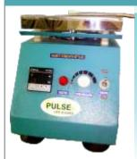
The PULSE Magnetic Stirrers are reliably designed to stir liquids in flasks. a two tier design provides stability and rigidity to the stirrer. digitalized temperature control provides high accuracy and reliability.
