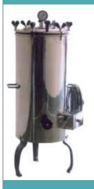
PULSE – ACV Autoclaves are made up of thick stainless steel (304) inner & the Outer body is made up of thick Mild Steel / Stainless Steel. The chamber is absolutely leak proof & can be operated at any selected point pressure upto 20 PSI, factory set at 15 PSI. Complete with pressure gauge, safety valve, and steam release valve.
