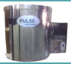
The PULSE Oil Baths are Double walled with inside made up of stainless steel & outside of mild steel sheet duly powder coated. The gap between the two walls is fitted with high – grade glass wool to minimize thermal loss. Temperature range from ambient 50 °C to 250 °C accuracy  $\pm$  2 °C. The temperature maintains to work on 220/230 volts A.C. supply.
