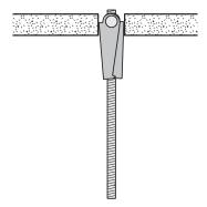
Drill a hole through the material. Use HSS-drill in plasterboards and other porous materials. Insert the Spring Toggle Anchor through the drilled hole. The toggle-wings will jump into place in the cavity
