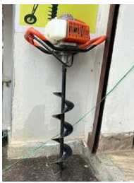
Manual Handle Earth Auger Drill Soil Digging
