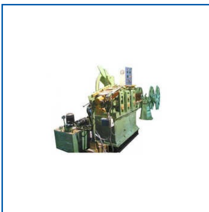
DOUBLE LAYER ROLL FORMING MACHINE
