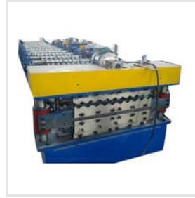
Corrugated Roof Rolling Machine
