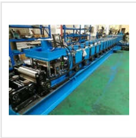
Automatic C Purlin Roll Forming Machine
