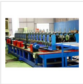
Cable Tray Roll Forming Machine
