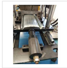
Rolling Shutters Making Machine
