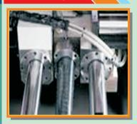
Bar Feeding assembly is fitted on Hardened Ground Hard Chrome Plated Bars for frictionless feeding of jobs by ball screw servo motor for repeatability within +/- 0.050mm equipped with FREE LIFTING mechanism helps to feed even bend bars, reduces the friction and scratch marks on the surface of bar during feeding, increases jaw liner life.
