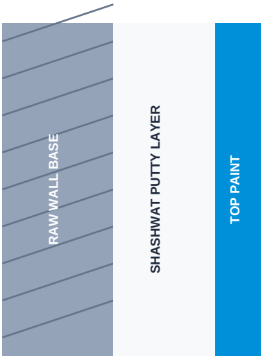
Figure 2: Layered Cross-Section Coating Application Profile
