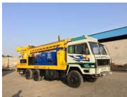
Truck Mounted Drill Rig
