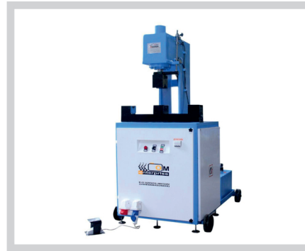
Scaffolding Pipe Straightening M/c.
