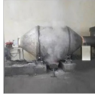
Lead Rotary Furnace
