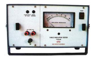
The function of this instrument is to measure the IR (Insulation Resistances) of the signaling pairwhen the signaling pairisun energized
