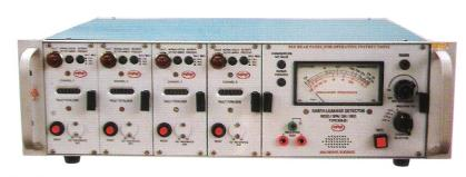
common for all channels while the visual indication is separate for each channel.
