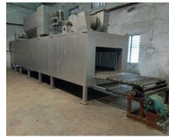
Core Oven Gas Fired
