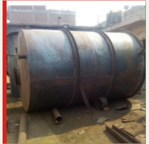
MS Sulfuric Acid Storage Tank
