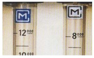
tube due to accidental ingress of tiny particles of dirt and this will usually remain unnoticed. This may mislead the operator, resulting in serious consequences. A rotating type of float will stop rotating in such a situation, thereby inviting the operator's attention to the improper functioning of the instrument: Reading is from the top level of the float.
