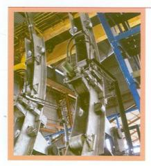
At the start of cast, the Rigid Dummy Bar head closes the mould. After start, the driven bar leads the hot strand through the cooling chamber and withdrawal & straightening unit. Rigid and sturdy construction of arc segments can be individually exchanged in case of damage. No obstacles exist (roller aprons, supports) in cooling chamber, therefore free access and perfect undisturbed spray pattern to hot strand is achieved. Restranding during casting of individual strand is possible.
