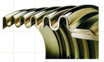
The value of the thrust force of bellows is usually calculated by multiplying the value of the effective cross section area by the value of the flow pressure of pipe
