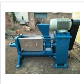
Municipal Waste Shredder
