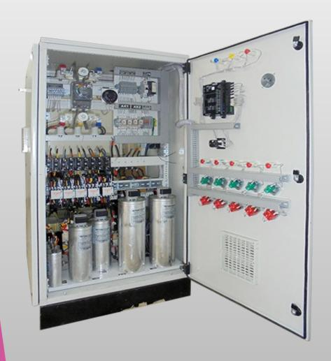
We can supplied Automatic Power Factor Control or APFC Panels are mainly used for the improvement of Power Factor. Power Factor is the ratio of active power to apparent power and it is a major component measuring electrical consumption. APFC is an automatic power factor control panel which is used to improve the power factor, whenever required, by switching ON and OFF the required capacitor bank units automatically.
