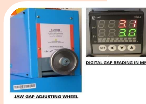
Digital reading showing actual gap between jaws in millimeter
