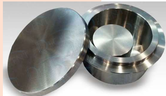
Hardened Steel Bowl Set Working Capacity 50 ml Bowl, Hammer, Lid, O-Seal
