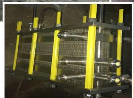
Primary Exchanger Material-Steel, Titanium
