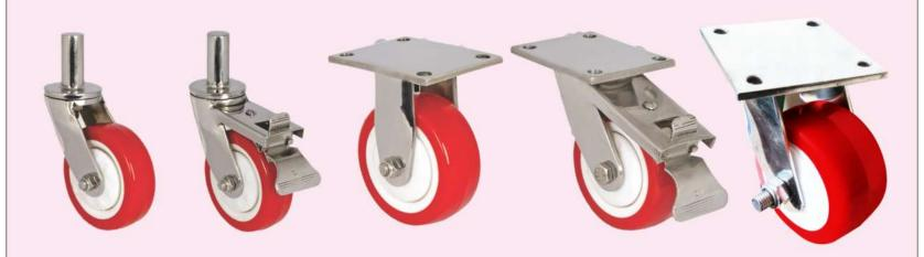
Stainless steel ss 304 with fabricated type this model contain with double bearing and body design arc welding and axle of wheel contain self locking nut
