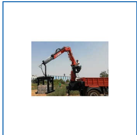
BRICK LOADER TRUCK MOUNTED CRANE
