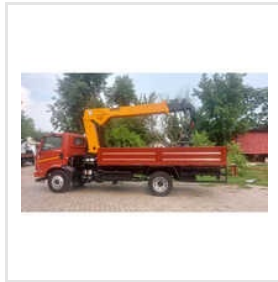
Stiff Boom Crane
