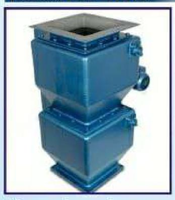
Suitable for discharging dry dust, powder, granules and fibrous materials from cyclones, filters, hoppers etc., whilst still maintaining an effective gas seal. The valve consists of two flaps connected by counterweights or spring loaded spindles, which are operated by means of a motor driven cam or pneumatic cylinder.
