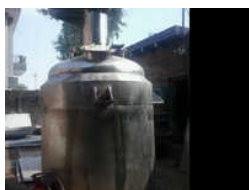
Stainless Steel Chemical Reactor
