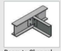
Beam to Channel
