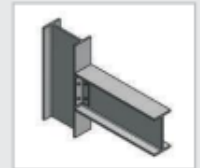
Beam to Beam
