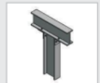
Beam Over Beam
