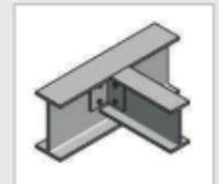
Beam to Beam
