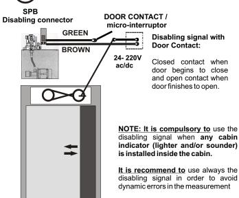
The SPB must continuously receive a blocking signal during all the time the lift is travelling, from the moment the doors are closing until the cabin gets on floor and the lift opens doors again. NOTE: Continuously. (Voltage 24-220Vac/dc)
