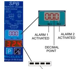
Note: The display remains switched off after 5 minutes of normal operation. Pressing any key the display value is visualised again.
