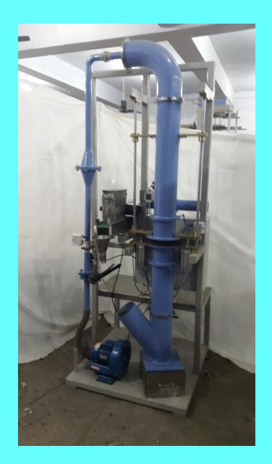
FILTER MEDIA TESTING BASED ON JIS VDI 3926 ISO 11057 ASTM 2008 STANDARD
