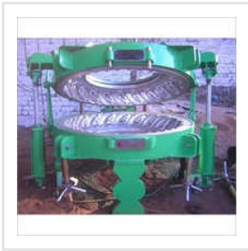
TYRE Resoling Plant
